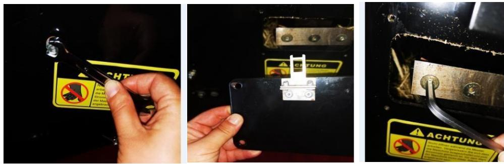
3. Remove one blade, rotate the impeller, and remove the second blade.
