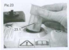
After approximately 150 hours of use, or every 3 months (whichever is sooner), the Fuel Tank Filter should be removed and cleaned thoroughly. The Fuel Tank Filter is displayed in Pic.23. As with cleaning the Air Filter, we recommend cleaning the Fuel Tank Filter with a water-based degreasing agent.
