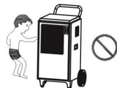
This unit use special electrical connection and outlet, don't use other extension wire or portable outlet.
